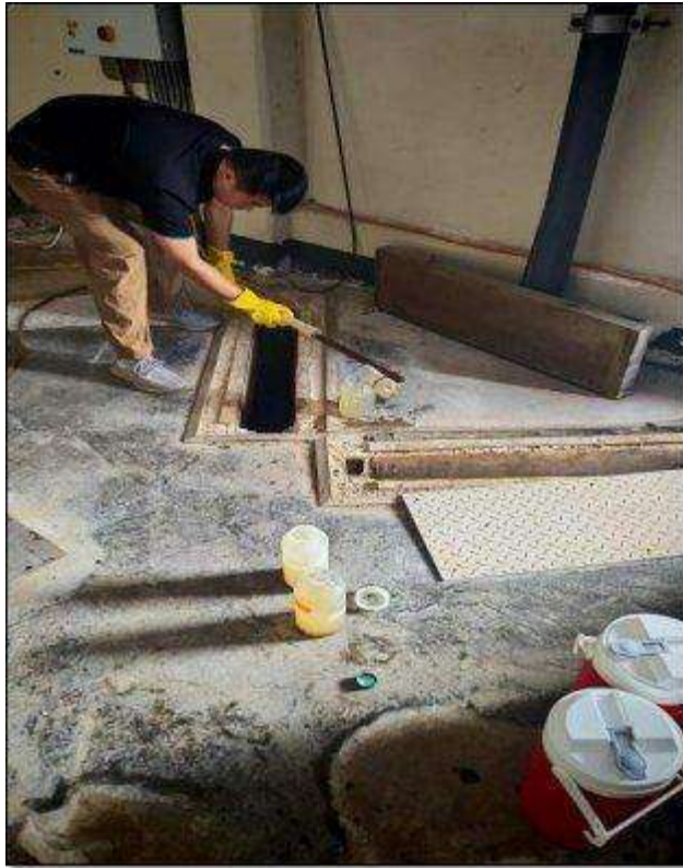
Figure 33: CRSEG's engineer collecting influent water sample at the SCSTP
