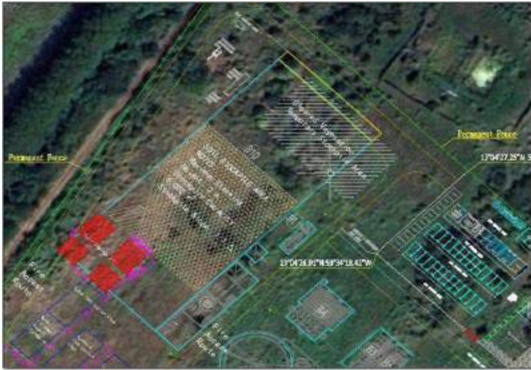
Figure 20: Cleared Vegetation and Topsoil Storage Location
