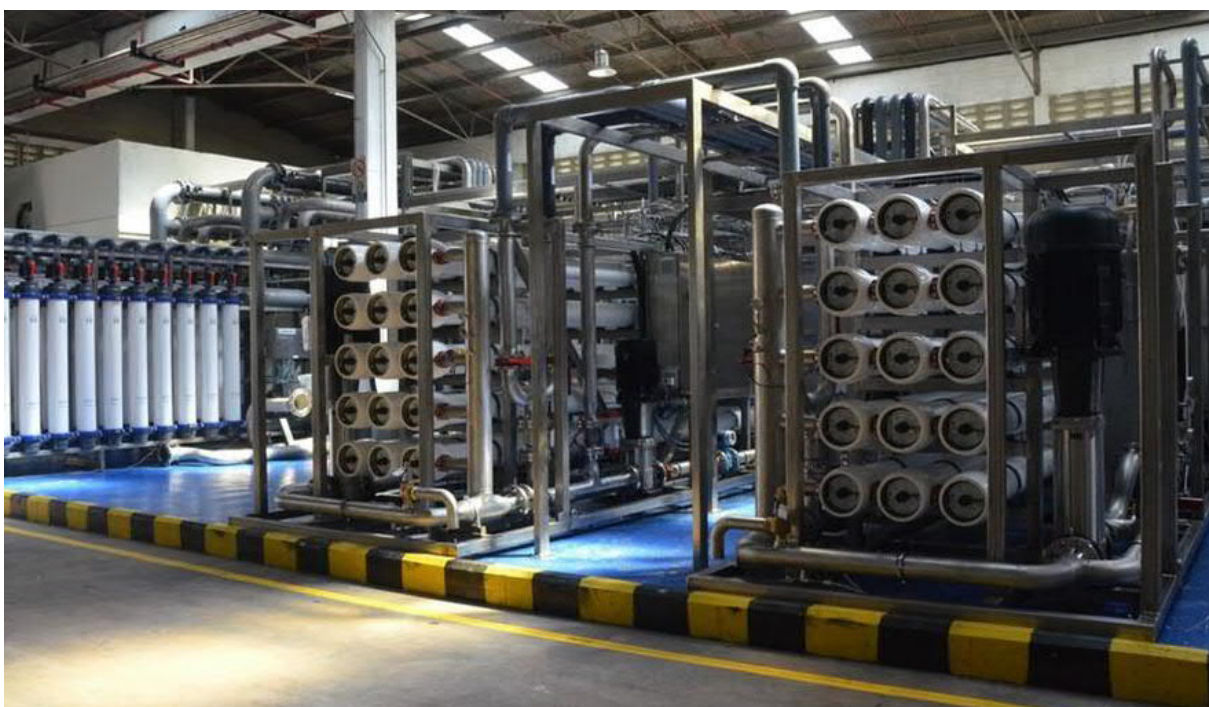
Figure 8-27: Example of RO skids (Desalitech)
