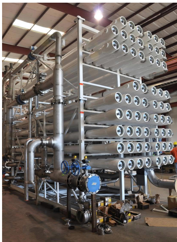
Figure 8-26: Example RO Skid (AECOM)
