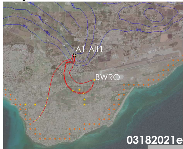
2 mgd RECHARGE at A1-A11 3 mgd WITHDRAWALS at BWRO
